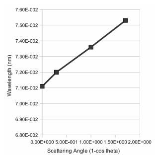
Figure 5: Compton Scattering for  $\lambda_1 = 0.0711 \text{ nm}$
