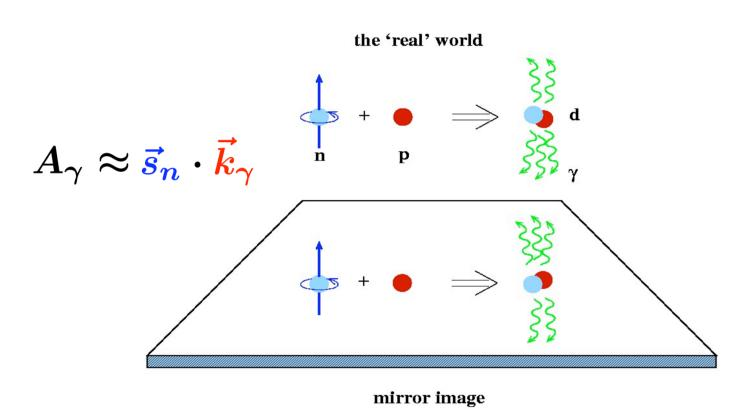
The goal of the NPDGamma experiment is to isolate the hadronic weak interaction (HWI) in neutron-proton capture, by observing a PV asymmetry in the emission of gamma rays. The gamma momentum is a vector, which changes direction under parity inversion. But spin is a pseudo-vector, and remains unchanged. Therefore, the correlation between these two quantities changes sign under parity inversion (violates parity).
