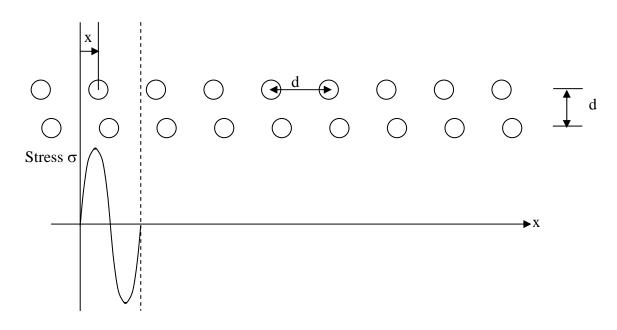
3. "Hooke's law":  $\sigma = Ce$ , but this linear relationship applies only to small strain e (or small displacement x). Since  $\sigma = A \sin (2\pi x/a) \Rightarrow \sigma = 2\pi A x/a$
