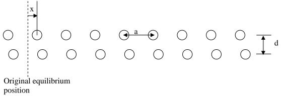
2. The force (and hence the shear stress) required is periodic because of the lattice periodicity. The magnitude of force can be modeled as sinusoidal. So,  $\sigma = A \sin (2\pi x/a)$  where a is the lattice constant or distance between two atoms in the same plane.
