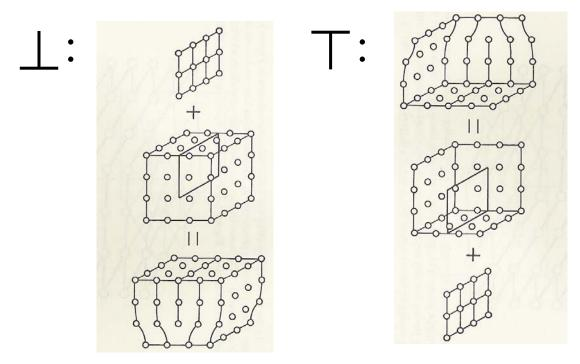
6. The lattice structure is near perfect except the line AA. The imperfection is concentrated around the line. For this reason, the line AA is known as the *line of dislocation*.
