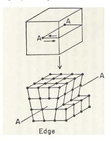
3. If the cut stops at line AA, and let the atoms at one side of the plane slip over a distance with respect to the atoms at the other side. The cut plane is also known as a *slip plane*.
