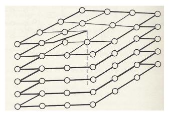
This is the reason why this is called screw dislocation. Again, there are two directions of screw dislocation – right hand and left hand. Note that the "handness" of a screw is independent of the direction at which it is looked at.
