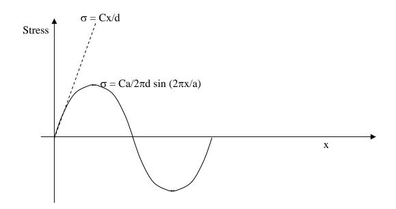
4. The amplitude  $\sigma_c = A = Ca/2\pi d$  is known as the critical shear stress at which the lattice becomes unstable and the top layer will slide into a new equilibrium position. For a ~ d, we have  $\sigma_c = C/2\pi$ . In other words, the critical shear stress is about 1/6 of the shear modulus.
