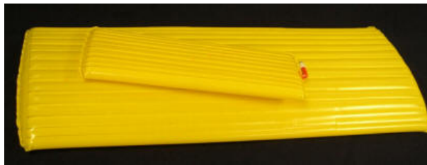
Figure 1. MIAV inflatable wings with bumpy NACA 4318 profiles courtesy of ILC Dover.
