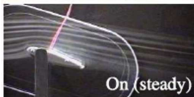
NACA 0015 airfoil at Re=217,000 , \alpha = 16^\circ
