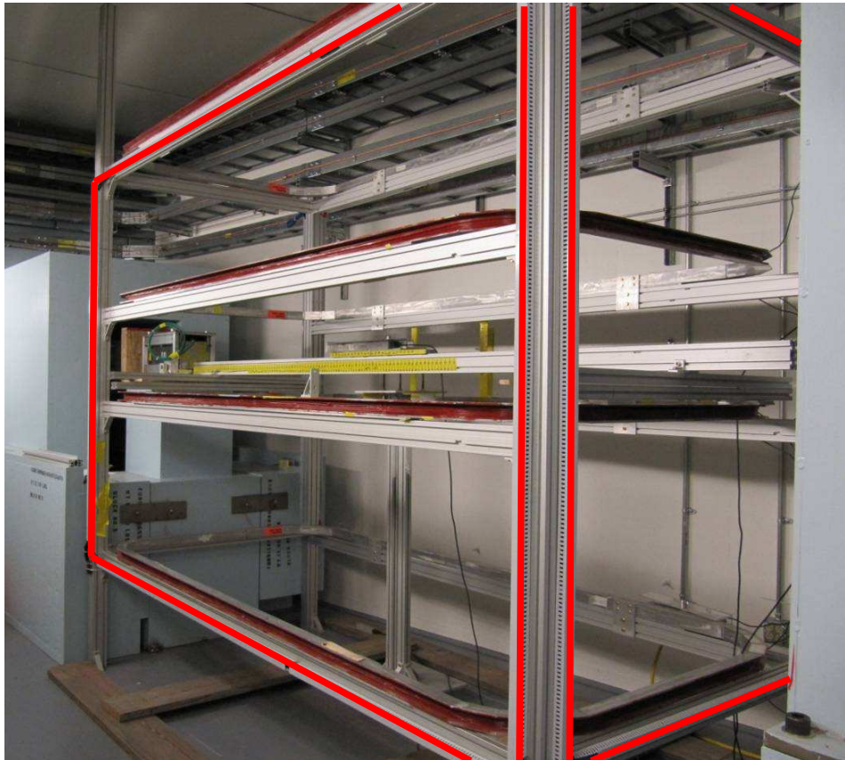
Figure 9: The coil stand in the cave; parts of the back and the right shim coil system are marked red.
