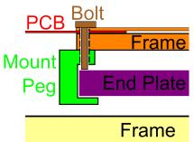
Using a variation of this peg design 4 pegs could be used to hold a 2 layer PEEK frame to sandwich the flexible kapton circuit into place spaced about the end plate.
