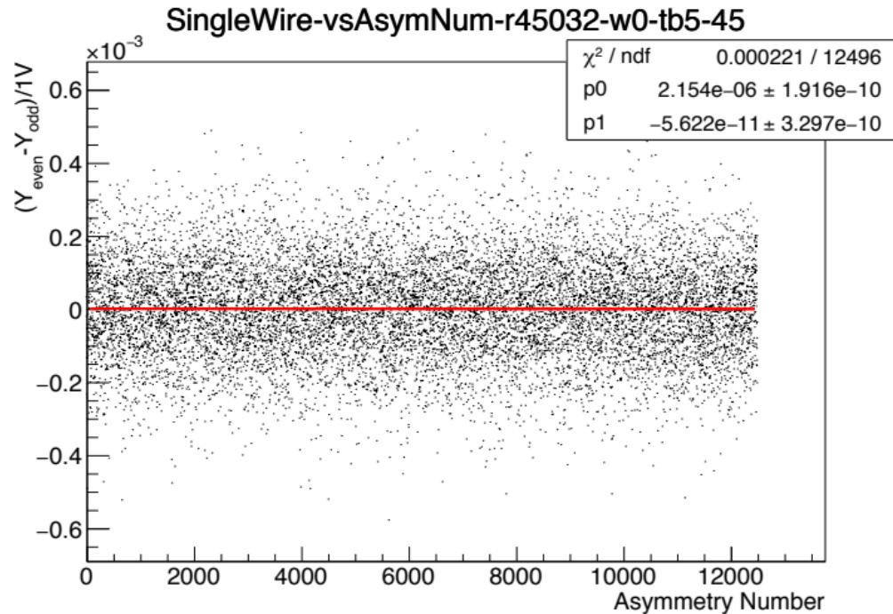
This plot shows the instrumental asymmetries and fitting parameters for one of the runs in the previous two plots.
