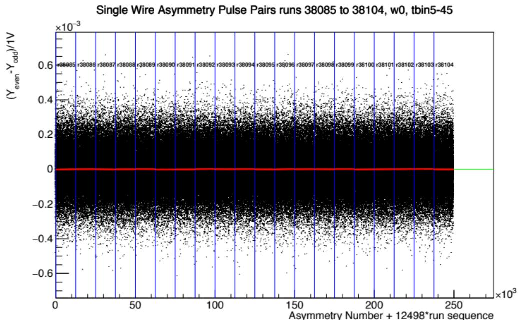
This plot shows all of the 12498 instrumental asymmetries that went into the average of the previous plot for a subset of the overall runs. Blue lines are separations between runs, the green line is a horizontal line at 0, and the red lines are fits made to each run.
