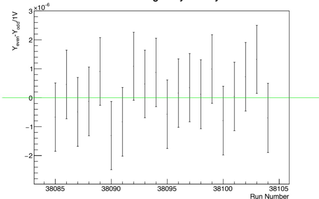
The run average and standard error of the instrumental asymmetry calculated for time bins 5-44.
