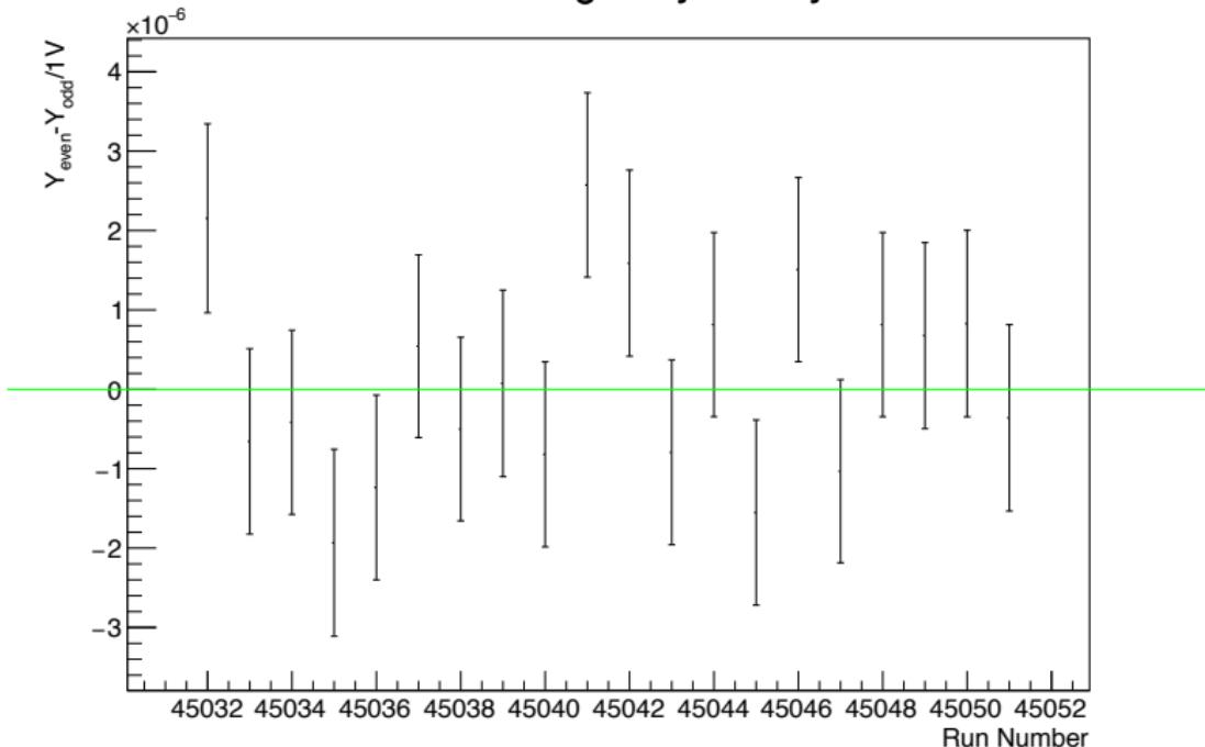
The run average and standard error of the instrumental asymmetry calculated for time bins 5-44.
