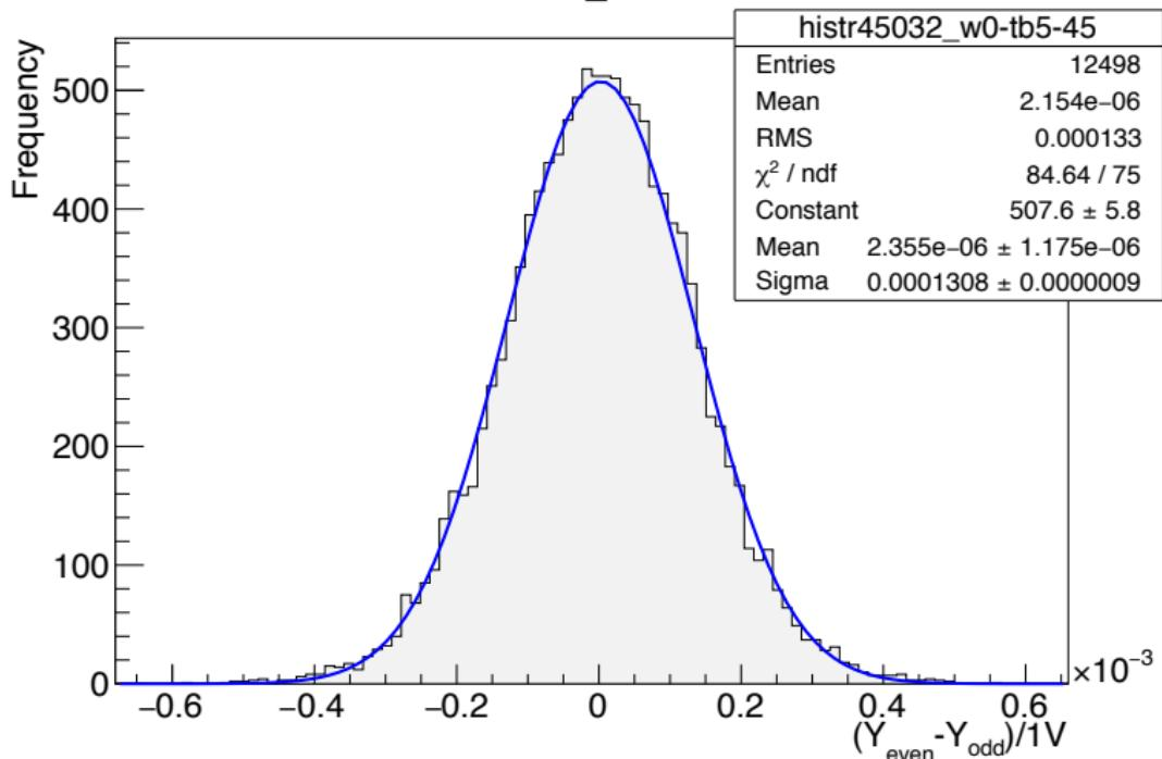
This is a histogram of the instrumental asymmetries calculated for one run that was graphed on the previous slide.
