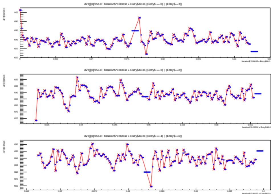
Red is original data points, blue interpolated data points. Periods of constant values between pulses was not preferred so this method was replaced by linear as described on the new slide.
