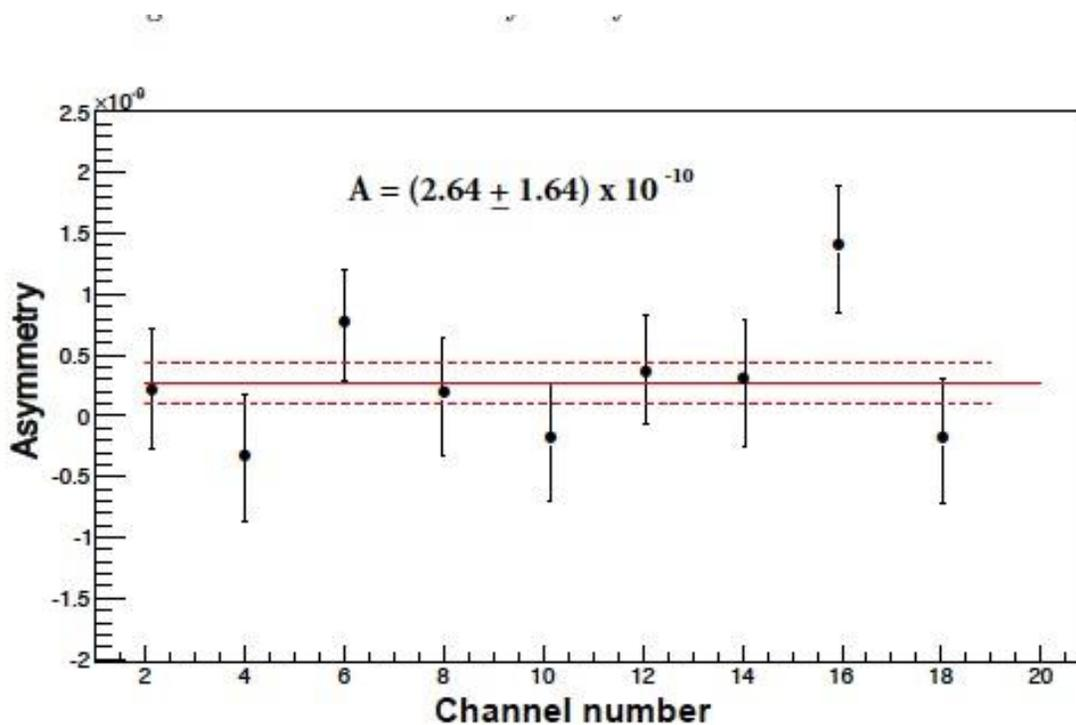
Figure 4.23: Instrumental asymmetry from different channels. Channel numbers have been reorganized in this plot.
