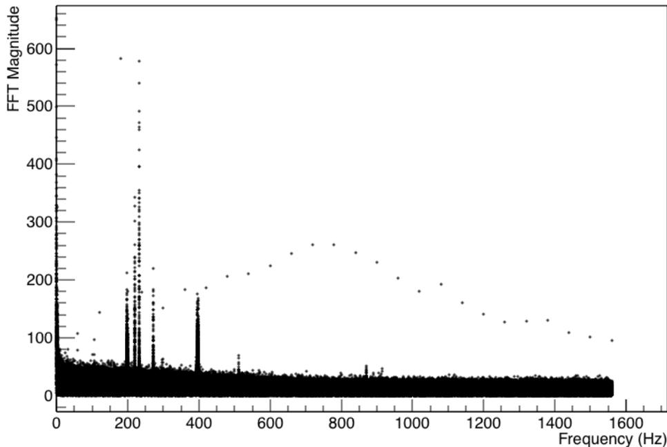
There is a flat component from 0 to 1550 Hz, a strong  $\delta$  function at 390 Hz, and a group of  $\delta$  functions between 200 and 270 Hz. We are interested in integrating the detector signal over some time interval within each frame. The time-domain operator is
