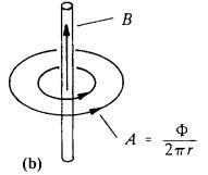
\* Coaxial cable, straight conductor
