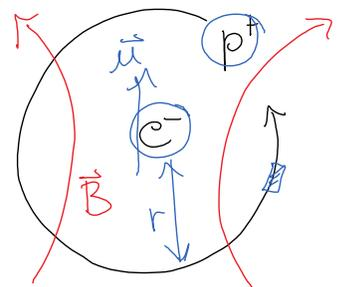
$$I_p A = \vec{\mu}_p = \gamma \vec{L} \Rightarrow I = \frac{\gamma}{A} L = \frac{e/2m}{\pi r^2} L$$
