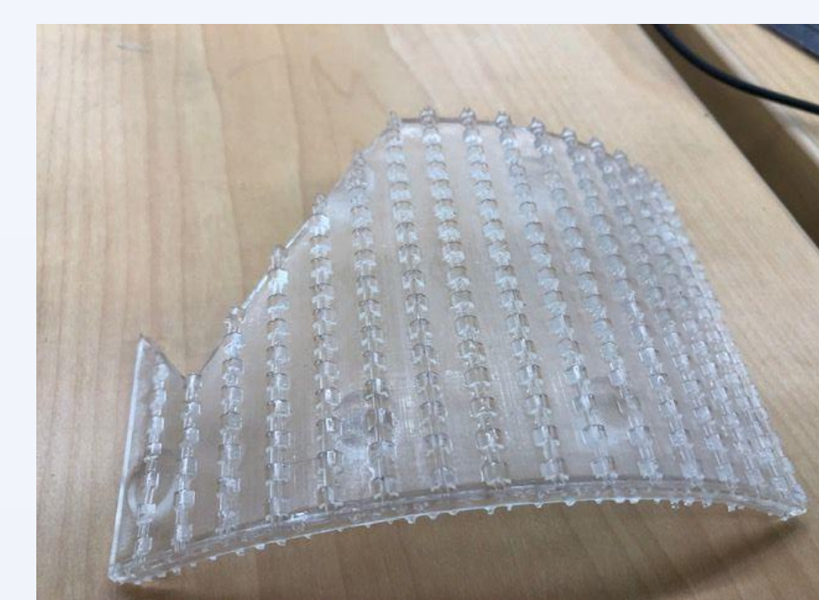
Figure 2: An example of a print breaking during the testing process.
