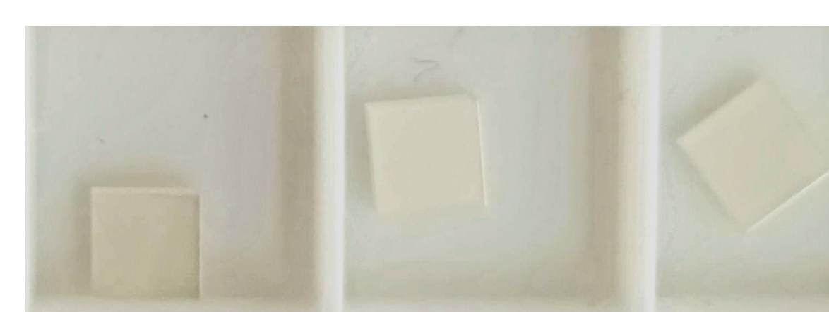
SrTiO 3 substrates before the 2 nd water leaching and annealing.
