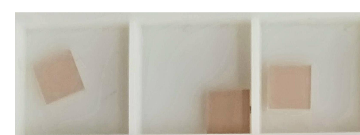
SrTiO 3 substrates after the 2 nd water leaching and annealing.
