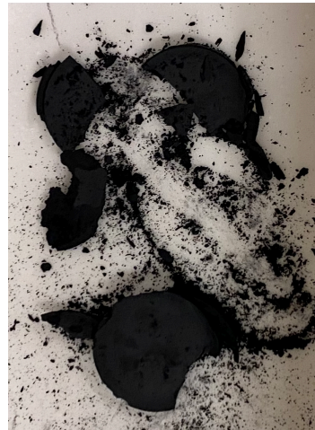
Figure 8: Broken Pellet of \text{SrCO}_3 + \text{Co}_3\text{O}_4 pressed at 36,000lbs. for 60 minutes.
