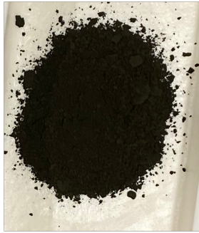
Figure 5: \text{SrCO}_3 + \text{Co}_3\text{O}_4 Before Calcination
