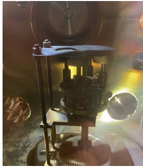
Figure 18: Pellet in PLD Chamber
