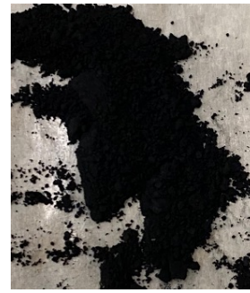
Figure 6: \text{SrCO}_3 + \text{Co}_3\text{O}_4 After Calcination
