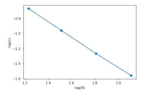
We ran these simulations with N=16, 32, 65, 128. The slope of the curve is approximately -1.01, which is above our predicted exponent, but memory overflow issues in the program kept us from simulating larger values of N.
