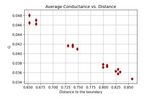
From the plot we can see that the conductance seems to depend on the distance. Also we see multiple points have the different conductance's for the same distance. The reason for this is that in a even numbered lattice there is no proper center as mentioned earlier. So our coordinates are not actually symmetric about the origin.
