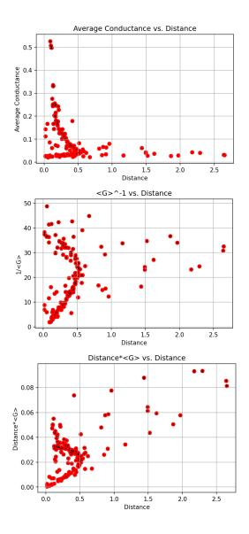
We can somewhat see a relationship, but evident from the plots the relationship between the conductance and the distance is not clearly evident. The function may be correct for coordinates in some vicinity in the lattice but is largely incorrect for the lattice. Further attempts will be made to find the correct function, but we must conclude this distance function is incorrect.
