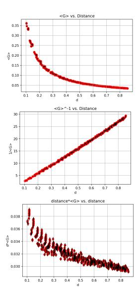
In this plot we can see the conductance relies on the distance more clearly. We can conclude that the conductance to the boundary depends only on this "distance".
