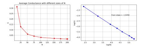
Our exponent is similar relative to the lattice with all conducting edges which is not too surprising because we expected similar behavior when the voltage point is placed at the origin: where it is the same distance from insulated boundary as the other conducting boundaries. Therefore because we saw this behavior in the previous case, we can reason that we can find a distance function that the conductance is dependent upon.
