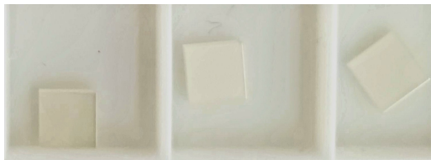
Figure 8: \text{SrTiO}_3 substrates before 1 st water leeching and annealing
