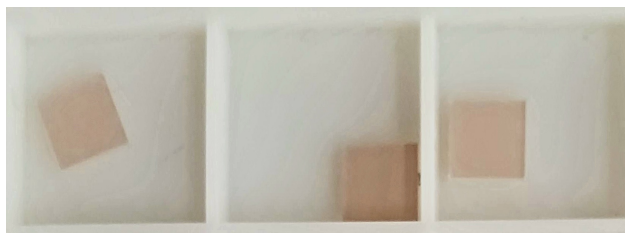
Figure 9: \text{SrTiO}_3 substrates after 1 st water leeching and annealing
