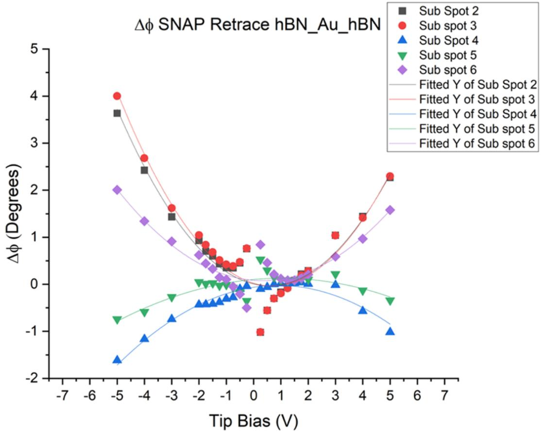
Figure 2:  $\Delta\varphi$  SNAP Retrace hBN-Au-hBN
