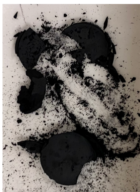
Figure 4: Pellet of SrCO 3 + Co 3 O 4 after in press at 36,000lbs. for 60 minutes.
