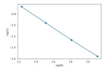
Dr. Straley and I ran some preliminary simulations with N = 17, 32, 65, 128. The slope of the curve is approximately -1.01, which is above our predicted t, but memory overflow issues in the program kept us from simulating larger values of N. After we fix that issue we plan to simulate lattices up to potentially N  $\sim$  1000.
