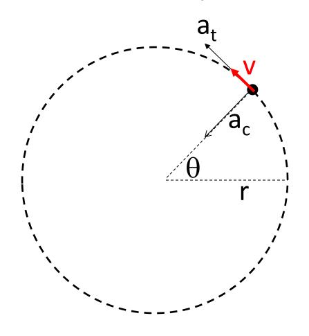
There will be a tangential acceleration (a<sub>t</sub>)causing the change in speed.
