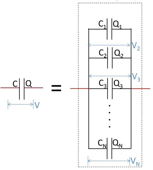
$$C = C_1 + C_2 + C_3 + \cdots + C_N$$
