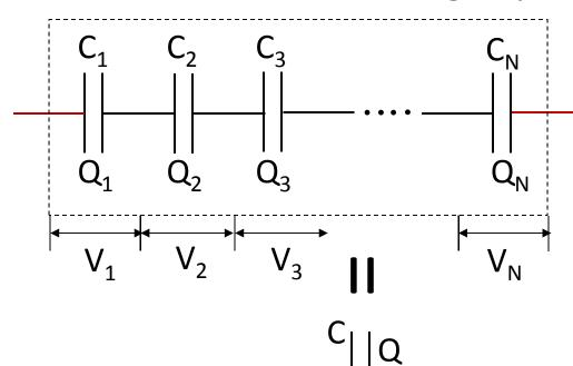
$$\frac{1}{C} = \frac{1}{C_1} + \frac{1}{C_2} + \frac{1}{C_3} + \dots + \frac{1}{C_N}$$
