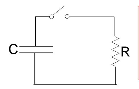
At t=0, capacitance is charged with a charge Q (initial condition).
