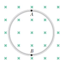
The flexible loop in the figure has a radius and is in a magnetic field of magnitude B. The loop is grasped at points A and B and stretched until its area is nearly zero. If it takes  $\Delta t$  to close the loop, what is the magnitude of the average induced emf in it during this time interval?
