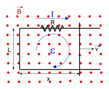
Motion emf is just a result of Lorentz force acting on the charge carriers due to the magnetic field.
