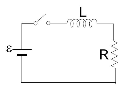
At t=0, inductor is uncharged and I=0 (initial condition).
