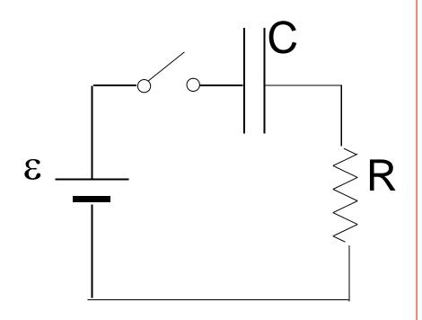
At t=0, capacitance is uncharged and Q=0 (initial condition).
