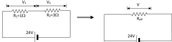
(d) If the two resistors are replaced with one, what should be the effective resistance R<sub>eff</sub> of the replacement?
