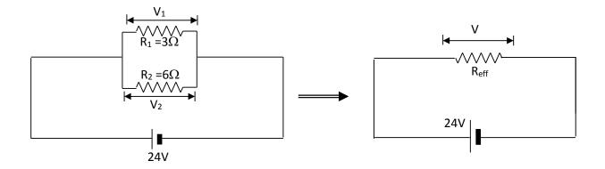
(d) If the two resistors are replaced with one, what should be the effective resistance  $R_{\text{eff}}$  of the replacement?
