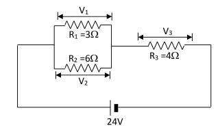
(a) What is the current through  $R_1$ ? What is the current through  $R_2$ ? What is the current through  $R_3$ ?
