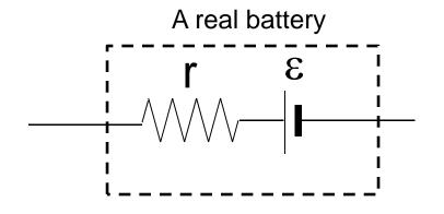
Electromotive force (emf  $\varepsilon$ ) is the maximum possible voltage the battery can provide between its terminal. You can think it like the voltage of an ideal battery with no internal resistance.
