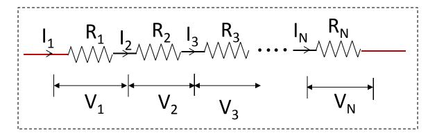
$$R_{eff} = R_1 + R_2 + R_3 + \dots + R_N$$
