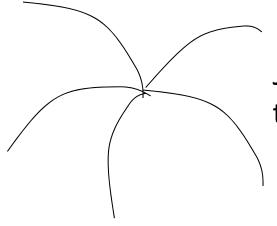
Junction formed by twisting many wires together.
