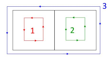
You can write Kirchhoff's voltage equations either for loops 1 and 2, or loops 1 and 3, or loops 2 and 3, but not 1, 2, and 3 because these three equations are dependent of each other.
