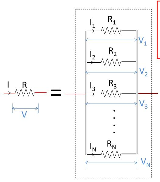
$$\frac{1}{R_{eff}} = \frac{1}{R_{1}} + \frac{1}{R_{2}} + \frac{1}{R_{3}} + \cdots + \frac{1}{R_{N}}$$
