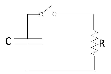
At t=0, capacitance is charged with a charge Q (initial condition).
