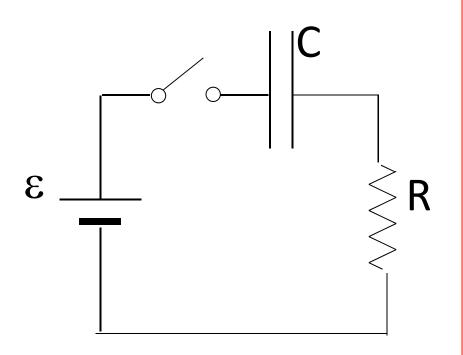
At t=0, capacitance is uncharged and Q=0 (initial condition).
