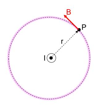
Want to calculate the magnetic field B at point P.
