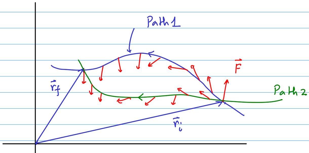
A conservative force is one for which the work done depends only on  $\vec{r}_i$  and  $\vec{r}_f$  and not on the path.
