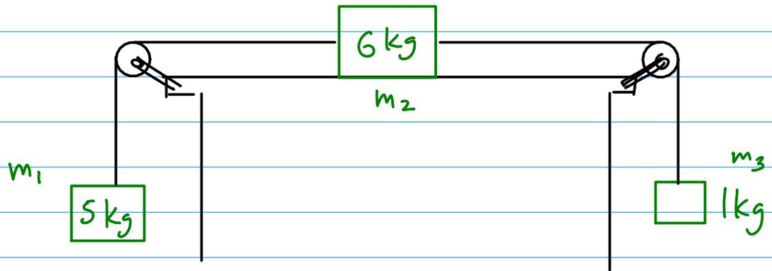
The 6 kg mass starts at rest and moves 1m to the left. Its final velocity is 1 m/s. What is  $\mu_k$ ?
