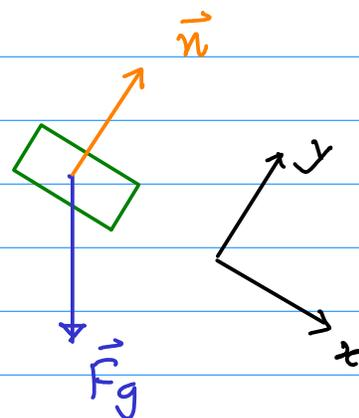
The block has both  $\vec{a}_r$  and  $\vec{a}_t$  because it speeds up as it slides down.
