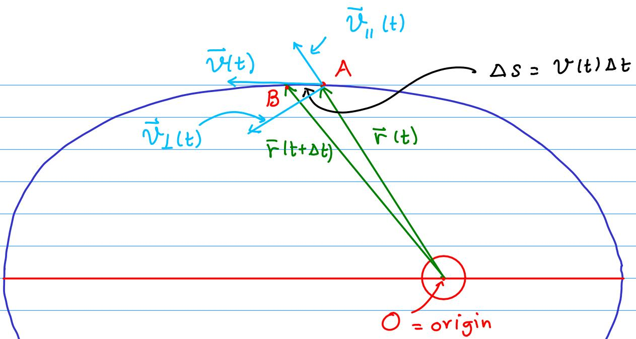
Between  $t$  and  $t+\Delta t$  the planet travels from A to B or from  $\bar{r}(t)$  to  $\bar{r}(t+\Delta t)$ .
