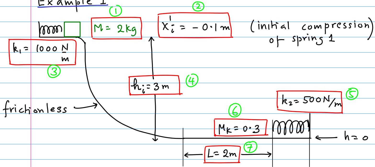
How far does spring 2 compress at its max compression?
